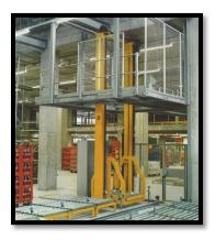
According to DC Velocity magazine, the ban extends to all kinds of VRCs. The material handling association MHI defines VRCs as power- or gravity-actuated lifts that move material vertically between two or more fixed
